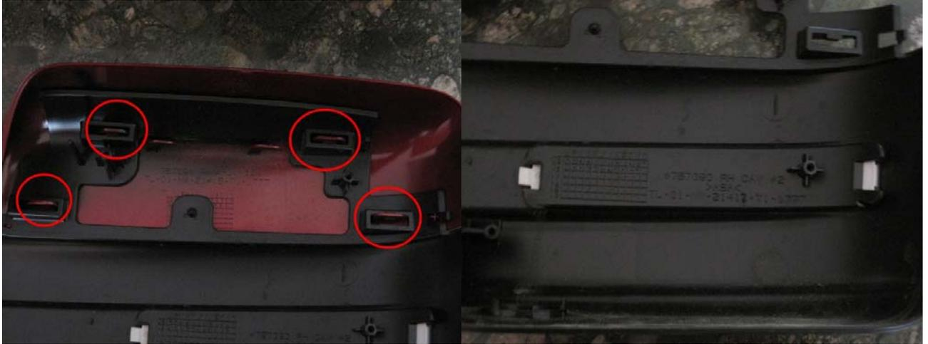
6. Now you can remove the reflector from the housing. Using a flat head screwdriver, gently pry the tab on the outside curved part of the reflector. NOTE: The driver mirror reflector tab on the door side is a fork shape instead of one solid tab.
