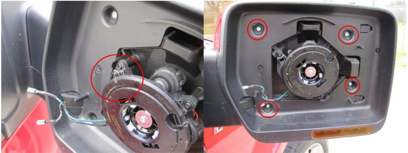
2. Once the mirror is free, very gently unplug the heated mirror wires (assuming your truck is equipped with them). Then remove the four (4) T15 torx screws. NOTE: If your heated mirror wires look fragile or frayed, we recommend you do not unplug them. You can still install RECON mirror lenses without unplugging these wires; however, you must be careful so you do not apply too much pulling pressure on these wires.
