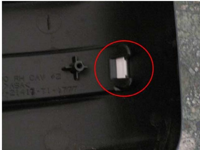
7. NOTE: This last step is ONLY if you are installing part # 264241Bk or CL which include LED turn signals &/or running lights. We recommend taking the strip of LED's and using it as a template to cut out the plastic with a Dremel tool using a cut-off wheel on it. Be sure not to run the Dremel too fast and don't cut too deep. Only cut deep enough to cut through the white plastic and then stop.
