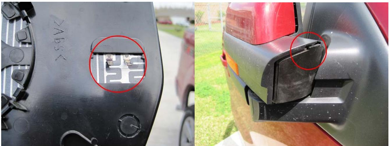
4. Now fold the mirror in towards the door of the truck so you can remove the front half of the housing. Start at the door side of the mirror and pry up as shown. Once you have this part up the housing should pop right off.
