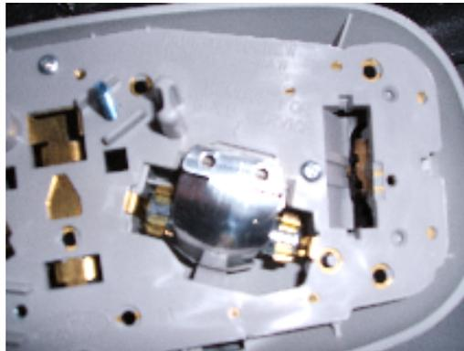
3) With the housing free, use a small flat head screwdriver to remove the right and left light reflector. Press the screwdriver against the small tab to release the reflector.
