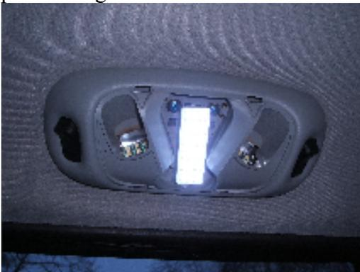
9) Rotate the LED spot lights so they face out the ports
